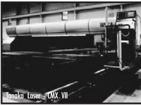
2 - Tanaka Laser - LMX VII • 6000 Watt • Table cut size 14' x 43', 14' x 54' • Cut up to 1.125"
