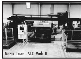
Mazak Laser - ST-X Mark II • 4000 Watt • Table cut size 78.7" x 157" • Cut up to 7/8" • Load material up to 3/4" • Fully automational
