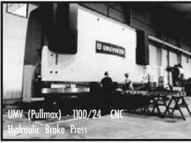
UMV (Pullmax) - 1100/24 CNC Hydraulic Brake Press • 1100 Tons • 6 Axis back gauge • CNC crowning • Bending length 24'4"
