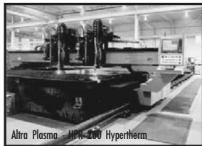
Altra Plasma - HPR 260 Hypertherm • Table cut size 14' x 44' • Plasma - 2 Heads - 1 1/2" Steel - piece capacity - 2 1/2" Steel - edge cut capacity • Oxy/Fuel torches - 4 Heads - 6" + cutting capacity
